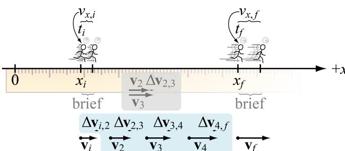
$$v_{x,i} + a_{x,\text{AVG}} \Delta t = v_{x,f}$$
